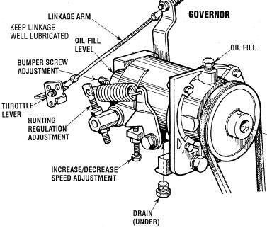
**4.** Periodically adjust the governor belt tension (see *DRIVE BELT ADJUSTMENTS*). Since belts stretch slightly, this stretching will, to some degree, affect the governor's action.
