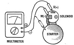
**NOTE:** Disconnect the wire from terminal M.
