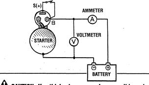
**CAUTION:** Use thick wires as much as possible and tighten every terminal securely. This is a solenoid shift-type starter which makes a rotating sound louder than that of a direct-drive type starter. When detecting starter rotation at the pinion tip, be careful not to come in contact with the pinion gear when it protrudes.
