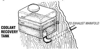
**NOTE:** Periodically check the condition of the manifold pressure cap. Ensure that the upper and lower rubber seals are in good condition and check that the vacuum valve opens and closes tightly. Carry a spare cap.
