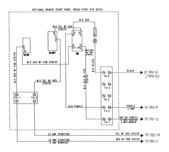
**NOTE:** Use #14 wire for all connections up to 100', increase to #12 wire for connections over 100'.
