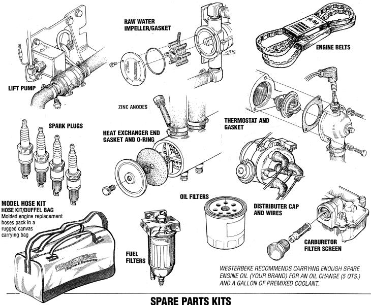
WESTERBEKE also offers two Spare Parts Kits, each packaged in a rugged, rust free toolbox. **KIT A** includes the basic spares.
