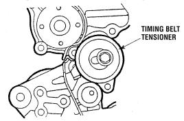
2. Fit one of the tensioner spring projections over the hooked portion of the belt tensioner and fit the tensioner onto the oil pump case.
