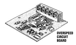
**CAUTION:** It is very important that the overspeed shutdown always be installed and functioning. Any tampering with the overspeed shutdown module, which would cause it to malfunction. could be a cause of injury should the generator's belt-driven governor fail and cause the generator to run away.
