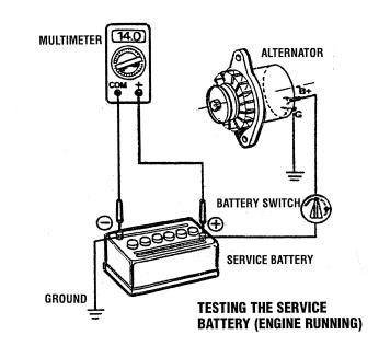
**CAUTION:** To avoid damaging the alternator diodes, do not use a high voltage tester (i.e. a megger) when performing tests on the alternator charging circuit.
